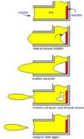
**Figure 9: Thermal Inkjet Printing (TIJ)**
