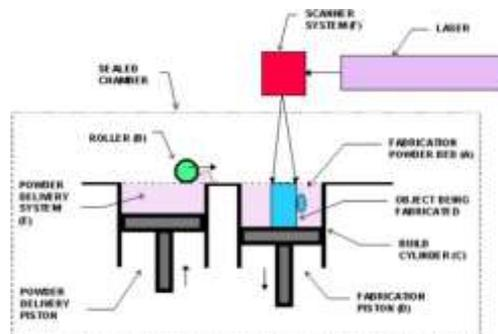
Figure 8: Selective Laser Sintering (SLS)
