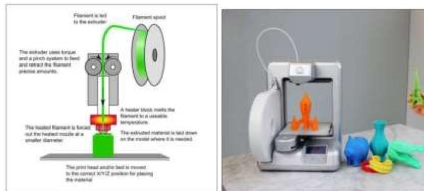
Figure 6: Fused deposition modelling (FDM)
