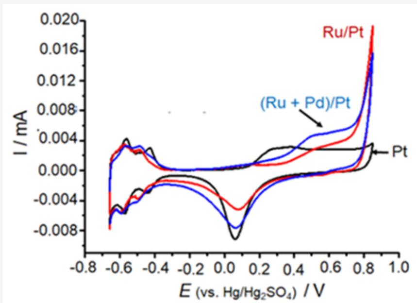
Figure 5.- Cyclic voltammetry of  $0.5 \text{ M H}_2\text{SO}_4$ ,  $10^{-4} \text{ M RuCl}_3$ ,  $(10^{-4} \text{ M RuCl}_3 + 10^{-4} \text{ M PdCl}_2)$ , at a Platinum electrode.  $\nu = 50 \text{ mV/s}^{-1}$
