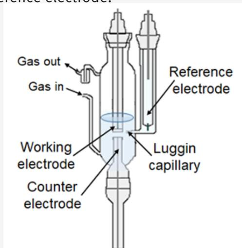
Figure 1.-Three electrode two compartment
