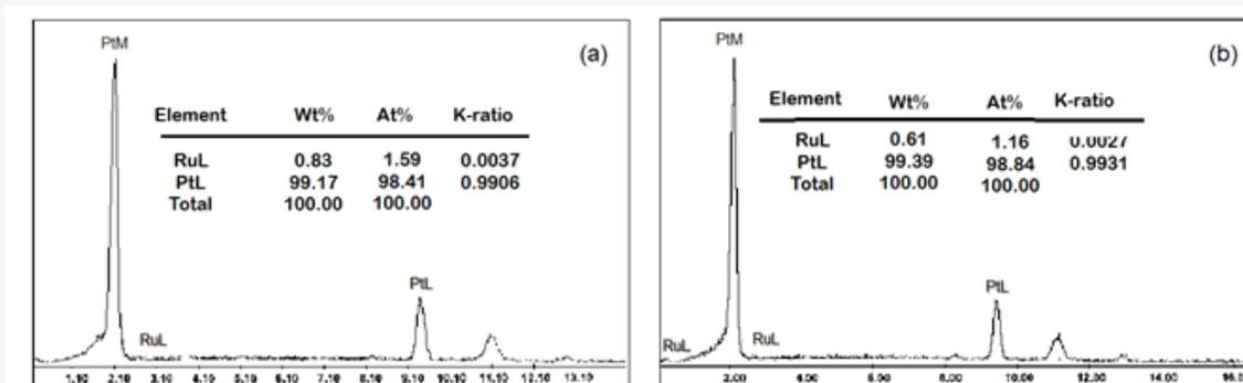
Figure 10.-EDX spectra of Ru deposits on Pt at different deposition potentials. (a) -550mV (b) -500 mV.  $[RuCl_3] = 5 \times 10^{-5} M$ .
