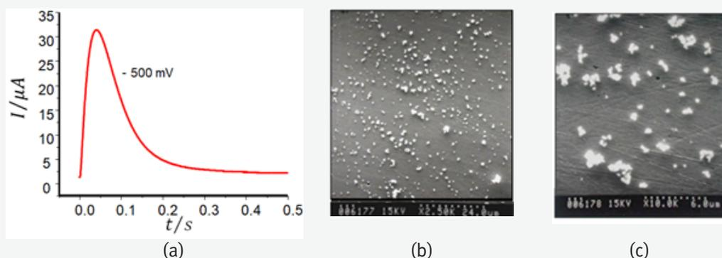
Figure 8.- (a) Current transient for Ru deposition on Pt at -500 mV, SEM of Ru deposits at different magnifications: (b) 2.50K, (c) 10.0 K
